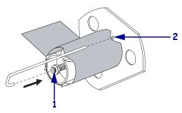
**b.** Rotate the spindle counterclockwise several turns to wind the media liner over the hook and remove any slack.
